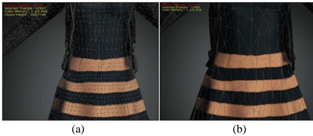
Figure 9. Illustrations of utilized Insta LOD polygon reduction approach for optimization of virtual characters. (a) 62,967 triangles Initially on a virtual character without polygon reduction with Insta LOD feature applied and (b) 37,085 triangles Initially on a virtual character without polygon reduction with Insta LOD feature applied.
