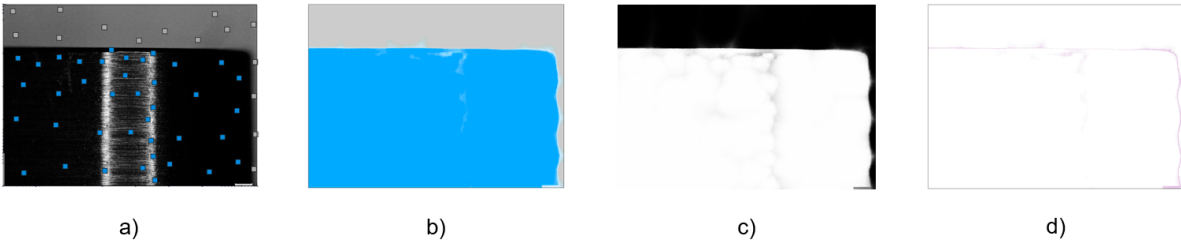
Fig. 4: a) Gray scaled image of cutting edge 3 with the user selected seed points for the cutting edge (blue) and the background (gray). b) Segmentation result color coded with the seed point's colors. c) Weight of cutting edge segment for each pixel (white: full ownership, black: not ownership). This result is forwarded in the visual industrial system pipeline. d) Uncertainty colorcoded with purple highlighting the pixels in the image that cannot be clearly segmented.
