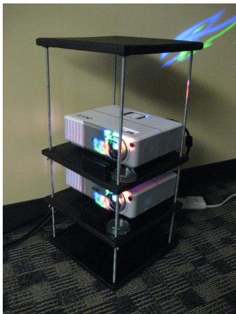
Figure 4. Set of projectors in a passive stereo configuration with polarization filters mounted in front of the lens.
