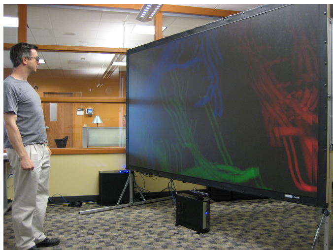
Fig. 3. Tracked user in front of the passive projection screen with the tracking computer and the Kinect sensor on top underneath the screen.
