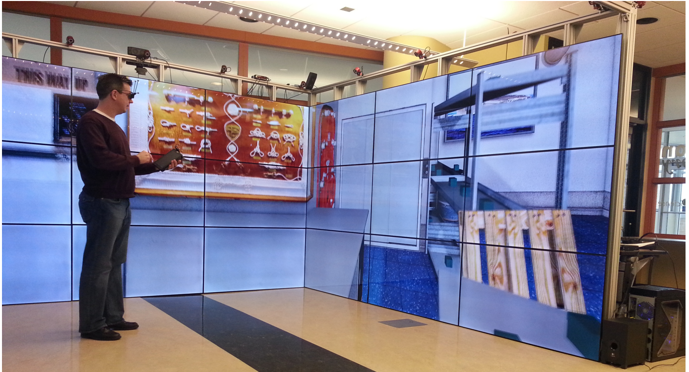
Fig. 6. Display infrastructure providing a fully immersive visualization virtual scenario.
