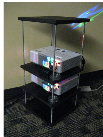
Fig. 2. Set of projectors in a passive stereo configuration with polarization filters mounted in front of the lens.
