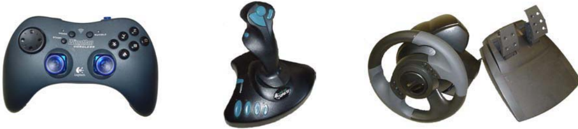
Figure 1: Different input devices supported by the exploration system: Logitech's WingMan Cordless Rumblepad (left), Primax' Raptor 3D joystick (center), and Microsoft's SideWinder force-feedback steering wheel with race car pedals (right).
