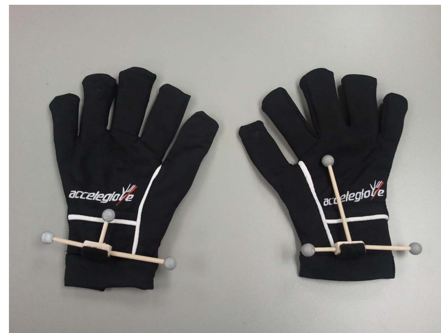
Data gloves used as input devices with attached marker spheres for optical tracking
