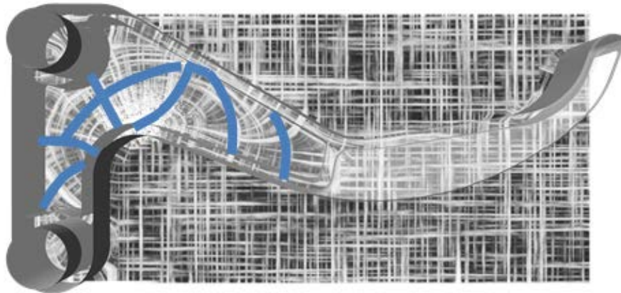
Fig. 40 Tensor fabric of the stress tensor in a planar cut through the CAD model. The engineer draw some lines manually to design rib support structures aligned with the tensor lines. These manual lines were the basis for the first new design. Two other drawings based on the same visualization led to the other two designs in our case study.
