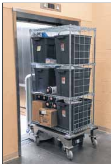
Eve and the other three robots can call for an elevator without pressing a button.
